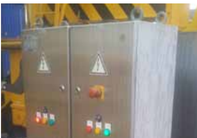
Ground mounted / Electrical interlock Power unit
